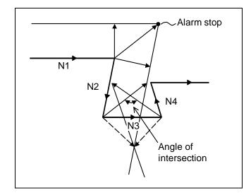
(c) When the program advance direction and the advance direction after compensation are reversed
