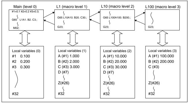
The status of the local variables appear on the setting and display unit. Refer to the Operation Manual for details.
