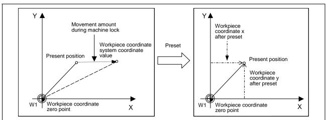
(6) When movement command is issued in machine lock state
