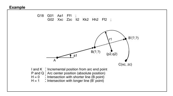
(3) Automatic calculation of arc-linear intersection
