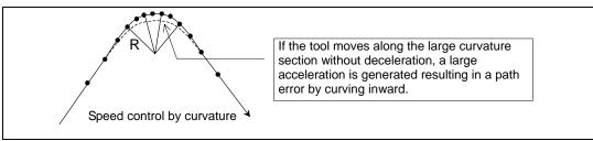
(Note) When a speed is set in "#2109 Clamp(H-precision)", clamp is executed at that speed. When the setting value is 0,clamp is executed with "#2002 clamp".
