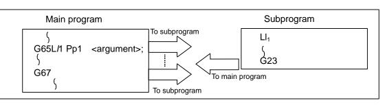
When the block with a movement command is commanded between G66 and G67, the movement command is first executed and then the designated user macro subprogram is executed. The number of times the subprogram is executed is  $\lambda 1$  times with each call. The argument is the same as for a simple call.
