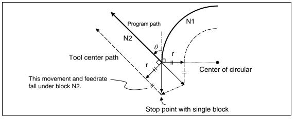
(2) If the arc is 360° or more due to the details of I, J and K at G40 after the arc command, an uncut section will occur.
