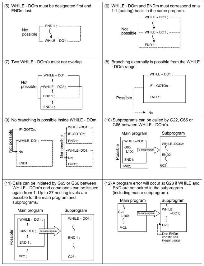
(Note) As the canned cycles G73 and G83 and the special canned cycle G34 use WHILE, these will be added multiple times.
