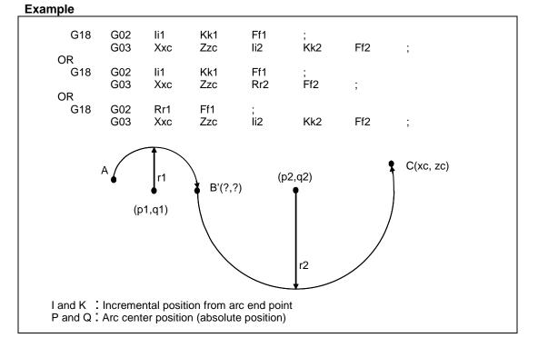
I and K are the arc center position (incremental position); distances from the start point in the first block or distances from the end point in the second block. P and Q (X, Z arc center position (absolute position)) can be commanded instead of I and K commands.
