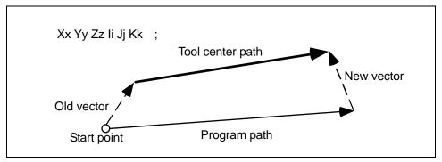
(4) Movement during the compensation: When there is no plane normal line vector command
