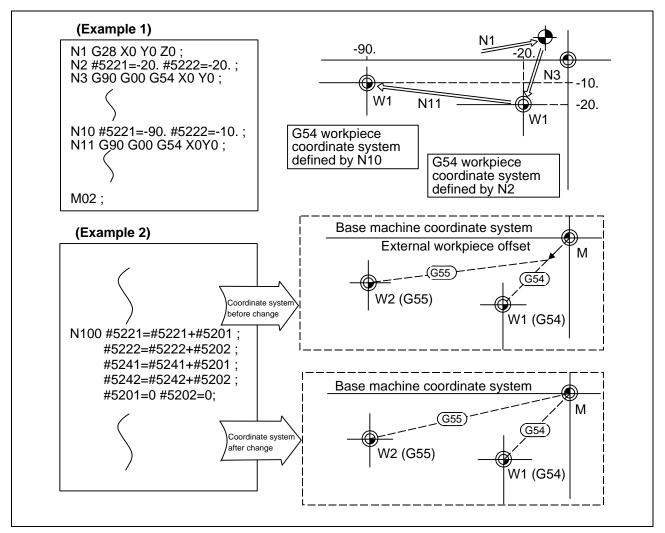
This is an example where the external workpiece offset values are added to the workpiece coordinate (G54, G55) system offset values without changing the position of the workpiece coordinate systems.
