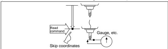
(4) The tool nose position where the tool compensation and other such factors are not considered is indicated as the end point position. The tool reference position with consideration given to tool compensation is indicated for the machine coordinates, workpiece coordinates and skip coordinates.
