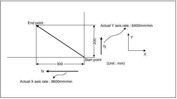
(Note 2) When parameter "#1086 G0Intp" is set to 1, the tool will move along the path from the start point to the end point at the rapid traverse rate of each axis.
