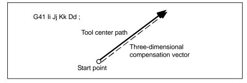
(3) Movement during the compensation: When there is a movement command and a plane normal line vector command
