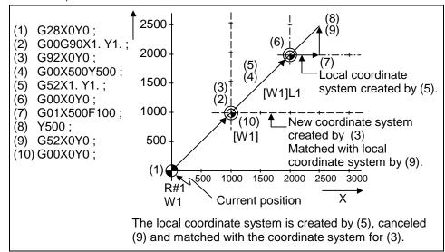
(Example 1) Local coordinates for absolute value mode (The local coordinate system offset is not cumulated)
