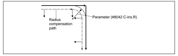
The stop point of the single block and block start interlock is as follows.
