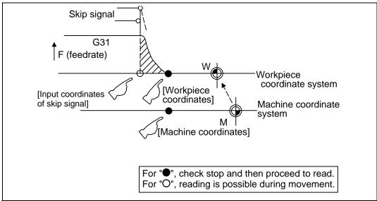
The position of the skip signal input coordinates is the position in the workpiece coordinate system. The coordinates in variable numbers #5061 to #5064 memorize the moments when the skip input signal during movement was input and so they can be read at any subsequent time. For further details, reference should be made to the section on the skip function.
