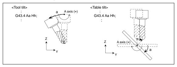
(b) Tool center point control type2 The program error (P33) will occur.
