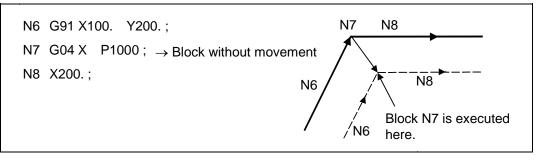
When 4 or more blocks without movement follow in succession or if there is a pre-read inhibit M code, the offset vectors are created perpendicularly at the end point of the previous block.
