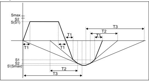
(ii)When synchronous tap changeover spindle rotation speed 2 < spindle rotation speed during return
