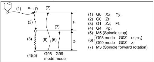
The operation stops at after the (1), (2) and (7) commands during single block operation.
