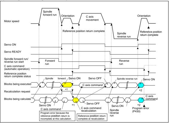
(Note) For axis commands, the reference position return complete is checked at calculation. Thus, when the C axis servo ON command and C axis command are continuous, the program error (P430) occur as shown above in \*2.
