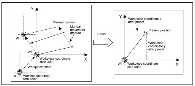
If manual operation is carried out when manual absolute is set to OFF, or if the axis is moved with handle interrupt, the workpiece coordinate system will be shifted by the manual movement amount.
