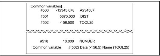
(Note) At the head of the variable name, do not use the characters determined by the NC for use in arithmetic commands, etc. (e.g. SIN, COS).
