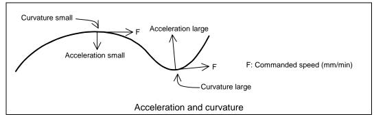
With the spline function, the high-accuracy control function is always valid. Thus, even if the curvature changes such as in this curve, the speed will be clamped so that the tolerable value of acceleration/deceleration before interpolation, which is calculated with the parameters, is not exceeded.
