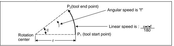
In this case, in order to make the cutting feed (linear feed) in the tool advance direction "fc"  $\,$  :
