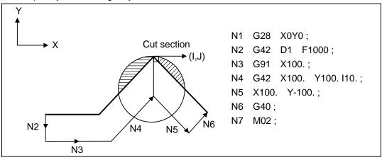
(3) The vectors differ for the G38 I \_J (K\_) command and the G41/G42 I\_J (K\_) command.
