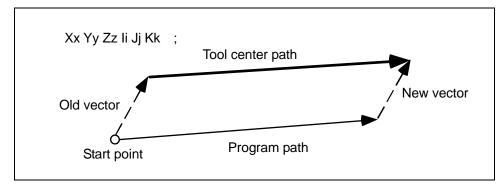
(5) Movement during the compensation: For arc or helical cutting
