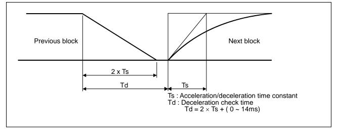
The time required for the deceleration check during cutting feed is the longest among the cutting feed deceleration check times of each axis determined by the cutting feed acceleration/deceleration time constants and by the cutting feed acceleration/ deceleration mode of the axes commanded simultaneously.
