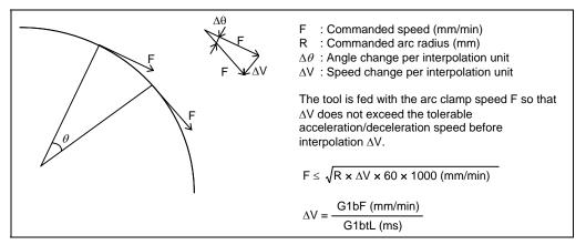
When the above F' expression is substituted in the expression expressing the maximum logical arc radius reduction error amount  $\Delta R$  explained in the section "a) Pre-interpolation acceleration/deceleration", the commanded radius R is eliminated, and  $\Delta R$  does not rely on R.
