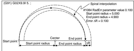
The parameter setting range is from 0.001mm to 1.000mm.
