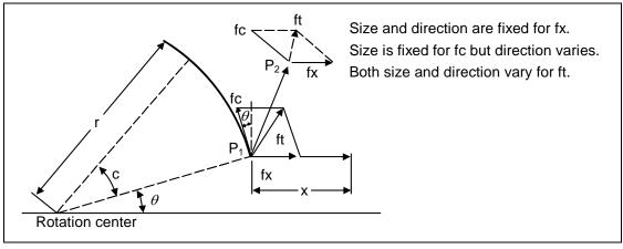
X-axis feedrate (linear speed) "fx" and C-axis feedrate (angular speed) " $\omega$ " are expressed as:
