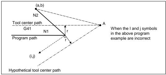
If the compensation vector obtained with point of intersection calculation is extremely large, a perpendicular vector will be created in the block before G40.
