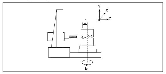
As programming can be carried out with a shape with which the side on the cylinder is developed, this is effective for machining cylindrical cams, etc. When programmed with the rotation axis and its orthogonal axis, slits, etc., can be machined on the cylinder side.
