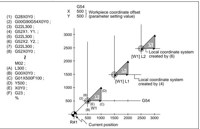
(Example 4) Combination of workpiece coordinate system G54 and multiple local coordinate systems
