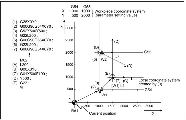
(Example 3) When used together with workpiece coordinate system
