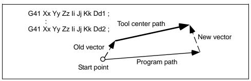
(Note 1) If I, J, K are not commanded in a block where the compensation amount is to be changed, the vector will be equivalent to the old vector. In this case, the modal will change, however, the compensation amount will change when I, J, K are commanded.
