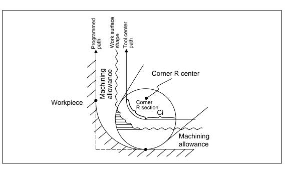
(1) The override set in the parameter is automatically applied at the deceleration range Ci and corner R section for inside offset with automatic corner R. (There is no angle check.)
