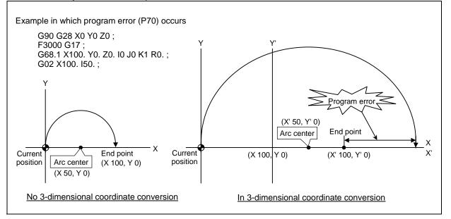
(2) For the arc in which the arc radius is specified with R, If the center coordinate has been deviated followed by the 3-dimensional coordinate conversion, a program error (P71 Arc center calculation disabled) will occur.
