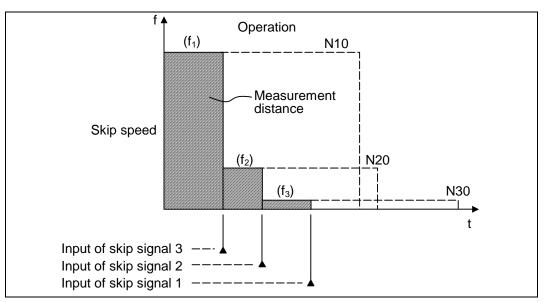
(Note 1) If skip signal 1 is input before skip signal 2 in the above operation, N20 is skipped at that point and N30 is also ignored.
