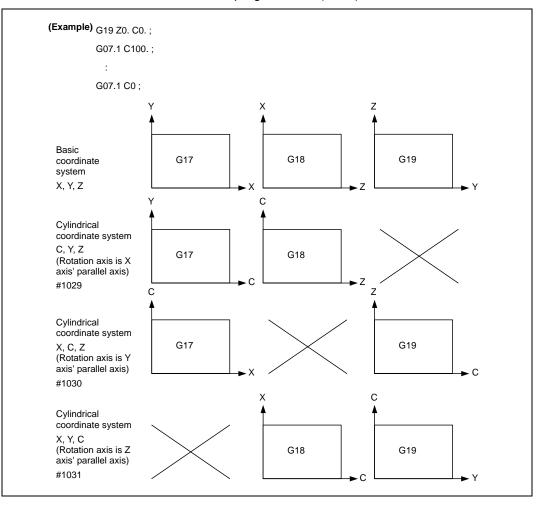
(Note) Depending on the model or version, the Z-C plane (Y-Z cylinder plane) will be automatically selected with G07.1 and G19.
