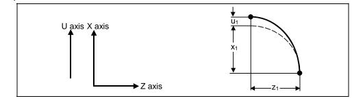
G18 G03 Xx<sub>1</sub> Uu<sub>1</sub> Zz<sub>1</sub> li1 Kk<sub>1</sub> Ff<sub>1</sub> ; ZX plane arc, U axis linear
