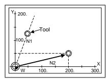
In the incremental value mode, the current position is the start point (0), and the movement is made only the value determined by the program, and is expressed as an incremental value.
