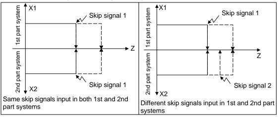
If the skip condition specified by the parameter "#1173 dwlskp" (external skip signals 1 to 8 are used for the specification) is met during execution of a dwell command (G04), the remaining dwell time is canceled and the following block is executed. Similarly, if the skip condition is met during revolution dwelling, the remaining revolution is canceled and the following block is executed.
