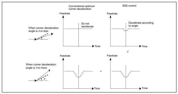
The length of the path direction recognized with SSS control can be adjusted with the machining parameter "#8091 StdLength". The range is increased as the setting value increases, and the effect of the error is reduced.
