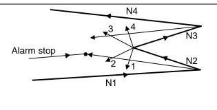
(ii) In a case such as that shown in the figure, the tool will move in the reverse direction at N2. Program error (P153) occurs after N1 execution.
