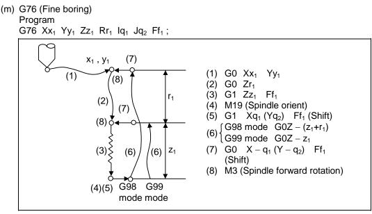
The operation stops at after the (1), (2) and (7) commands during single block operation. When this command is used, high precision drilling machining that does not scratch the machining surface can be done.
