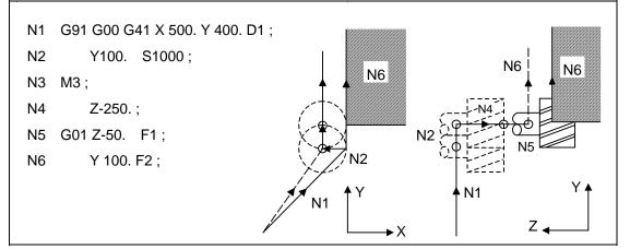
The movement is correctly compensated as the same direction as the N6 advance direction is commanded in N2.
