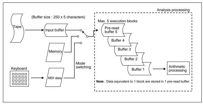
The input buffer has a memory capacity of 250 x 5 characters (including the EOB code).
