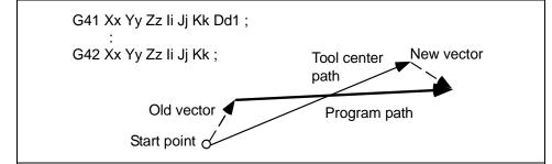
(Note 1) If I, J and K are not commanded in a block where the compensation direction is to be changed, the vector will be equivalent to the old vector and the compensation direction will not be changed.
