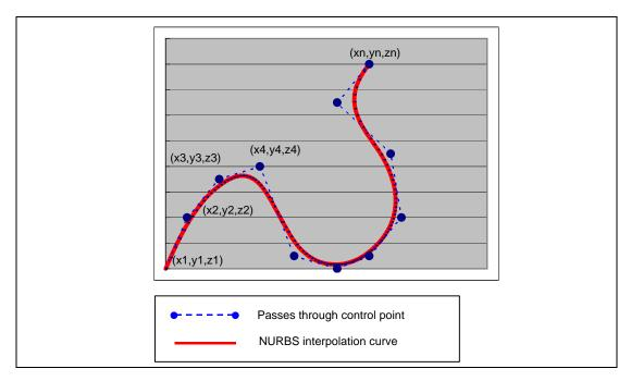
(Note) If an exclusive knot is commanded after NURBS interpolation immediately, NURBS interpolation mode is active again.
