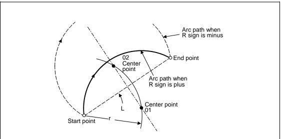
The following condition must be met with an R-specified arc interpolation command:
