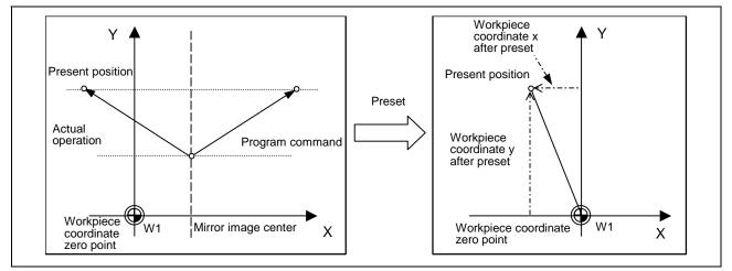
If operation is carried out with mirror image, only the NC internal coordinates are used as the program command coordinates. The other coordinates are the present position coordinates. This function sets the NC internal coordinates as the present position coordinates.
