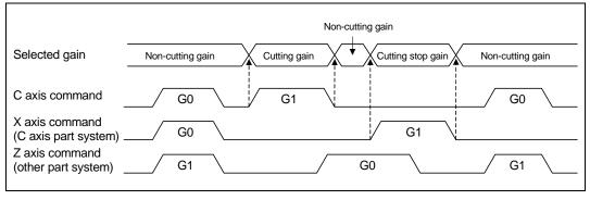
(Note 1) The cutting feed of other part systems does not affect the C axis gain selection. (Note 2) There are 1st to 3rd cutting gains, which are selected with the ladder.
