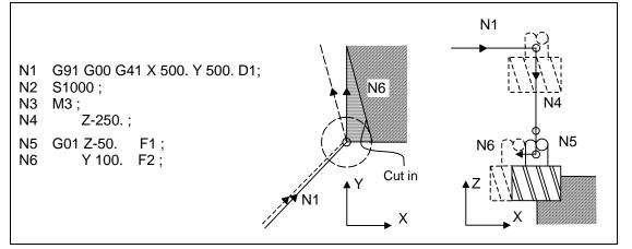
In this case, the four blocks N2 to N5 do not have a command in the XY plane, so when the N1 compensation is started, the program cannot be read to the N6 block.
