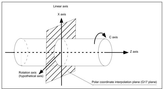
This is effective for cutting a notch section on a linear section of the workpiece diameter, and for cutting cam shafts, etc.
