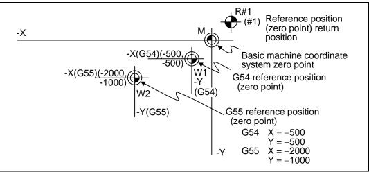
(6) The offset settings of workpiece coordinate systems can be changed any number of times. (They can also be changed by G10 L2(L20) Pp1 Xx1 Zz1.)
