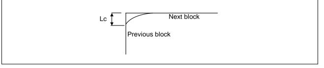
To eliminate corner roundness, set the value as small as possible to servo parameter "#2224 SV024" and perform an in-position check or assign the dwell command (G04) between blocks.
