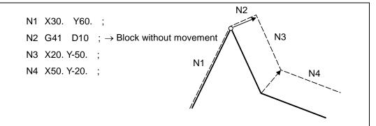
If four or more blocks containing no move command continue or if there is a pre-read inhibit M code, no compensation vector is generated.
