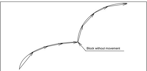
(d) When a block markedly longer than other blocks exists in spline function If the ith block length is Li in the spline interpolation mode, and it is given as "Li > Li - 1 × 8" or "Li > Li + 1 × 8", the block will be interpreted as a linear section, and the spline mode will be temporarily canceled. However, if the parameter "#8030 MINUTE LENGTH" is set to "-1", the mode will not be canceled.
