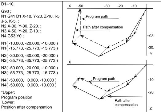
(b) For the incremental command, the axis will move by the amount obtained by subtracting each axis vector from the incremental movement amount. (The compensation amount is temporarily canceled.)
