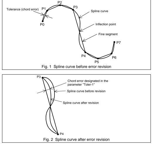
When the above conditions are satisfied, the spline curve will be revised so that the error between P3-P4 in Fig. 2 is within the designated value.
