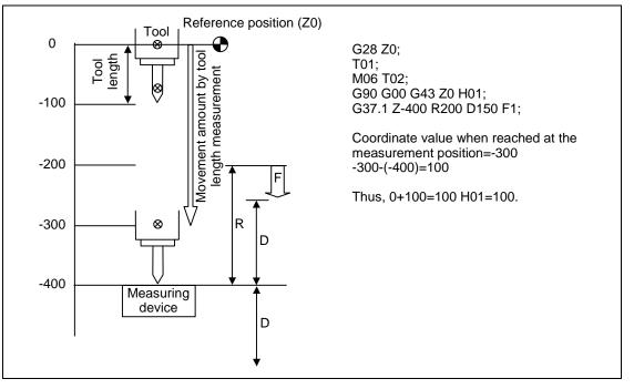
(Note) A new measurement is applied when the current tool length compensation amount is zero. Thus, length will be compensated whether or not length dimension by tool compensation memory type and length wear are differentiated.
