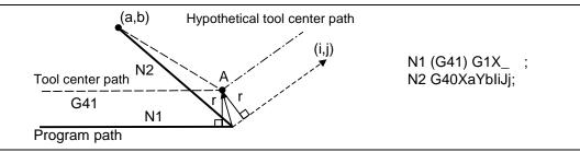
In this case, the point of intersection will always be obtained, regardless of the compensation direction, even when the commanded vector is incorrect as shown below.
