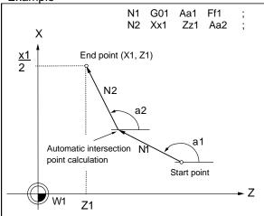
a: Angle (°) formed between straight line and horizontal axis on plane. The plane is the selected plane at this time.
