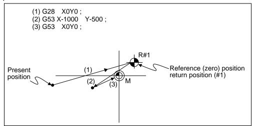
When the first reference position coordinate is zero, the basic machine coordinate system zero point and reference (zero) position return position (#1) will coincide.
