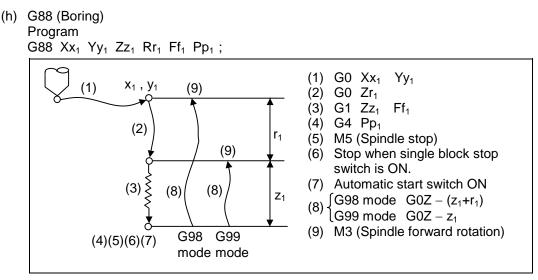
The operation stops at after the (1), (2), (6) and (9) commands during single block operation.
