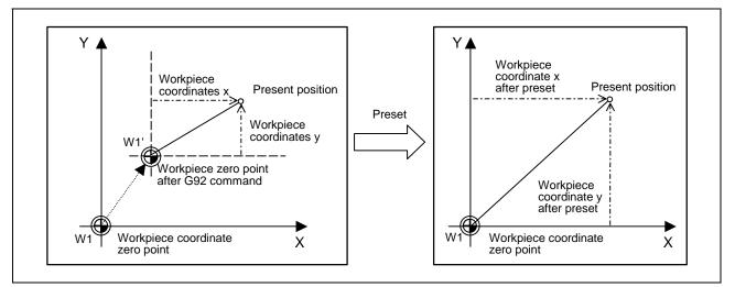
The workpiece coordinate system shifts with the G92 command, and the distance between W1' and the present position is set as the present position of the workpiece coordinate system. This function returns the shifted workpiece coordinate zero point to W1, and sets the distance from W1 to the present position as the workpiece coordinate system's present position. This is valid for all workpiece coordinate systems.
