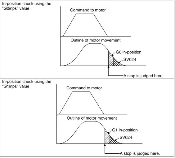
When the SV024 value is larger, the in-position check is completed when the error amount is smaller than the SV024 setting value.
