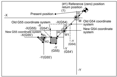
(Note) The workpiece coordinate system will shift each time steps (3) through (5) are repeated. The reference position return (G28) command should therefore be issued upon completion of the program.
