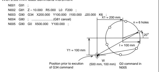
As shown in the example, the tool position after the G34 command is completed is over the final hole. When moving to the next position, the coordinate value must be calculated to issue the command with an incremental value. Thus, use of the absolute value mode is handy.
