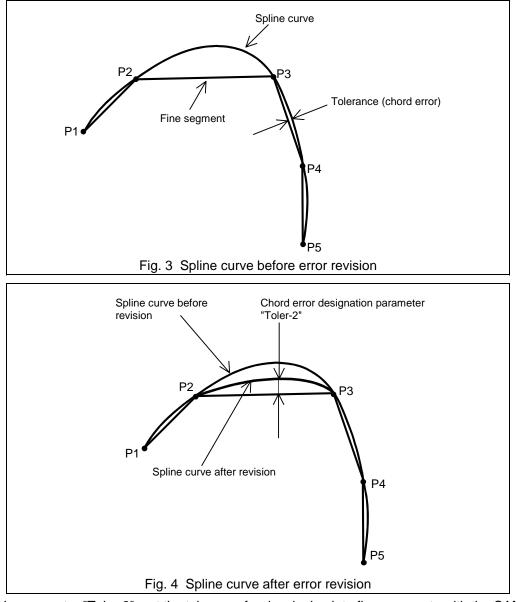
When the above conditions are satisfied, the spline curve will be revised so that the error between P2-P3 in Fig. 4 is within the designated value.
