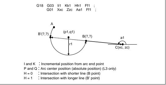
(4) Automatic calculation of linear-arc contact
