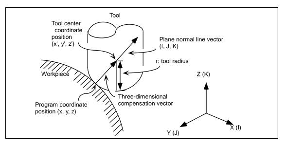
As shown above, the tool is moved to the tool center coordinate position (x', y', z') which is offset by the tool radius "r" in respect to the program coordinate position (x, y, z) following the plane normal line vector (I, J, K).
