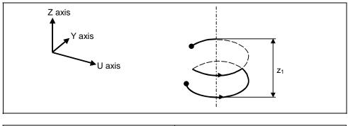
G17 G03 Uu<sub>1</sub> Yy<sub>1</sub> Zz<sub>1</sub> Ii<sub>1</sub> Jj<sub>1</sub> P2 Ff<sub>1</sub>; UY plane arc, Z axis linear
