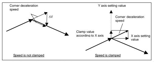
Note that the speed is controlled with the optimum corner deceleration speed in the following cases.
