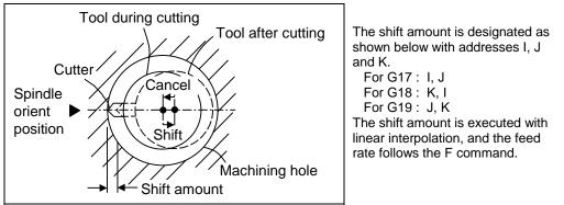
Command I, J, and K with incremental values in the same block as the hole position data. I, J and K will be handled as modals during the canned cycle.
