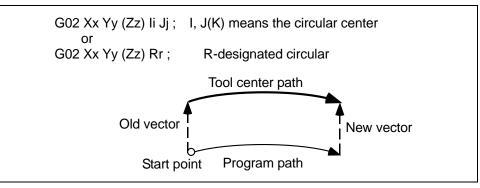
(Note) The center coordinate will not shift during the circular or helical cutting. Thus, when I, J, K are commanded with the vector as below, the program error (P70) will
