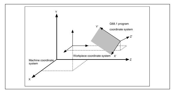
When the G68.1 command is issued, the zero point is shifted by the command value (x, y, z) in respect to the current local coordinate system. A new G68.1 program coordinate system rotated by the designated rotation angle "r" in respect to the commanded rotation center direction (i, j, k) is created.
