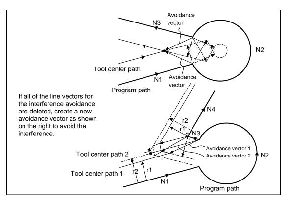
In the case of the figure below, the groove will be left uncut.
