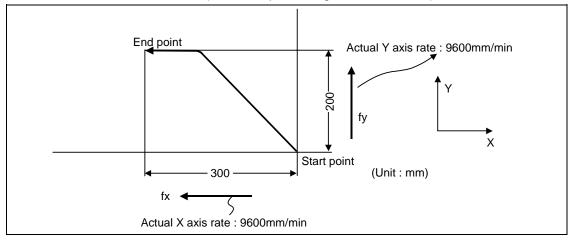
(Note 3) The rapid traverse rate for each axis with the G00 command differs according to the individual machine and so reference should be made to the machine specifications.
