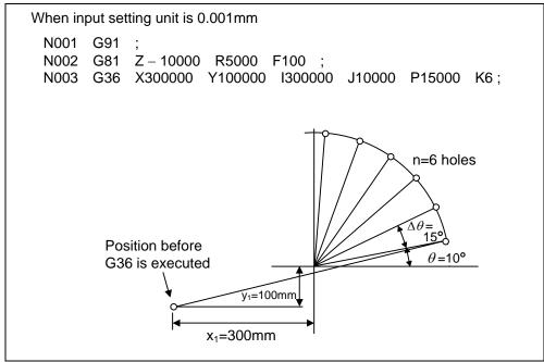
(Note 1) If an address other than the selected plane's vertical axis, horizontal axis, G, N, I, J, K, H, O, P, F, M, S or 2nd miscellaneous function is issued in the same block as the G36 command, a program error (P32) will occur.
