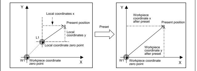
The local coordinate system is set with the G52 command, and the program commands, etc., are issued with the local coordinate system.
