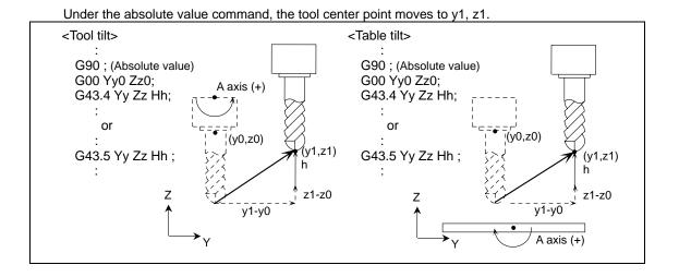
(b) Tool center point control type2 The rotary axis moves toward the commanded workpiece surface vector (I,J,K) direction along the movement command issued.
