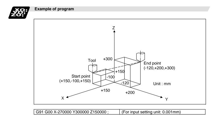
(Note 1) When parameter "#1086 G0Intp" is set to "0", the path along which the tool is positioned is the shortest path connecting the start and end points. The positioning speed is automatically calculated so that the shortest distribution time is obtained in order that the commanded speeds for each axis do not exceed the rapid traverse rate.
