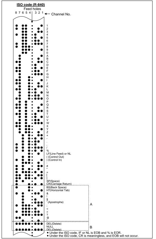
Code A are stored on tape but an error results (except when they are used in the comment section) during operation.
