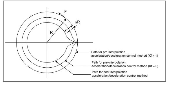
(Note) If the machine vibrates when Kf is set to 1, Kf must be lowered or the servo system must be adjusted.
