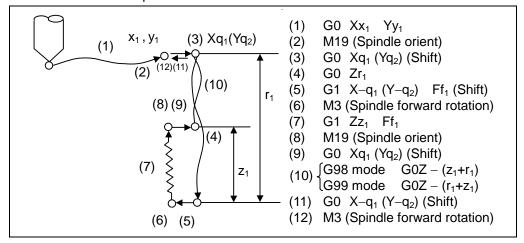
The operation stops at after the (1), (4), (6) and (11) commands during single block operation.
