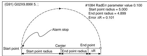
(b) Spiral interpolation in the direction of the commanded end point results when error ∆R is less than the parameter value.
