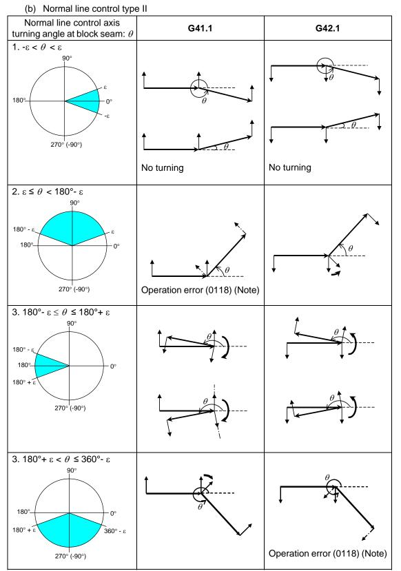
(Note) Turning operation in the command direction is performed in the inside of the workpiece. Therefore, an operation error will occur.
