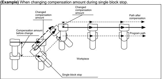
(Note 3) When changing compensation amount, the compensation amount corresponding to the actual compensation No. will be changed. However, when executing the NC reset or tool length compensation in the direction of tool axis cancel (G44), the compensation amount will be returned to the original.
