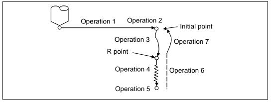
Operation 1: This indicates the X and Y axes positioning, and executes positioning with G00.
