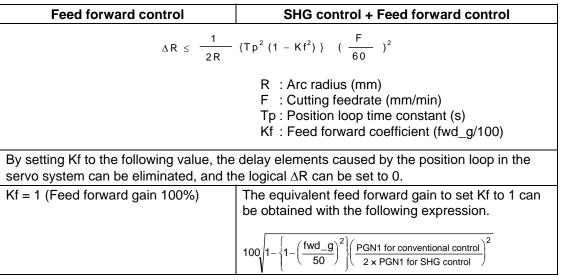
The feed forward gain can be set independently for G00 and G01.
