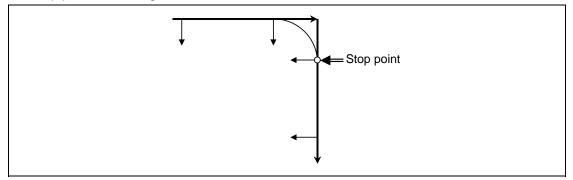
The stop point of the cutting start interlock is as follows.
