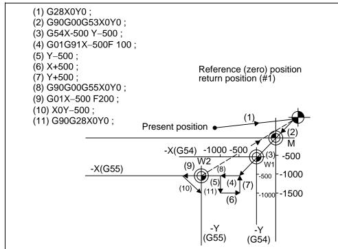
**(Example 3)** When workpiece coordinate system G54 has shifted (-500, -500) in example 2 (It is assumed that (3) through (10) in example 2 have been entered in subprogram 01111.)
