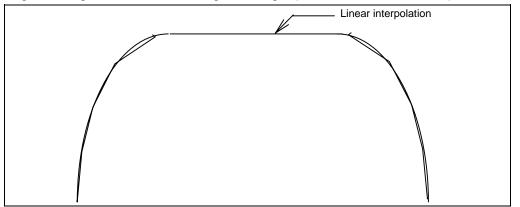
If the #8030 is set to "-1", the spline interpolation will not be canceled according to the block length.
