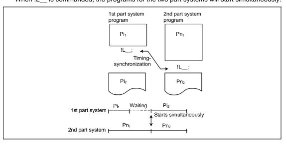
(2) The timing-synchronization command is normally issued in a single block. However, if a movement command or M, S or T command is issued in the same block, whether to synchronize after the movement command or M, S or T command or to execute the movement command or M, S or T command after synchronization will depend on the parameter (#1093 Wmvfin).
