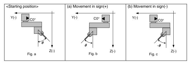
\*The position in which the tool center-point-side rotary axis or the table base-side rotary axis is 0.
