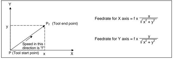
(Example) When the feedrate is designated as "f" and linear axes (X and Y) are to be controlled:
