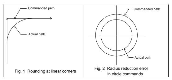
This function uses the following fix functions to minimize the increase in machining time while reducing the shape error.
