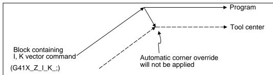
(5) Automatic corner override will not be applied when intersection calculation cannot be executed.
