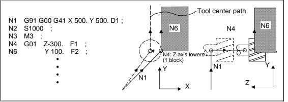
With this program, at the start of the N1 compensation the program will be read to the N6 block. The relation of N1 and N6 can be judged, and correct compensation can be executed as shown above.
