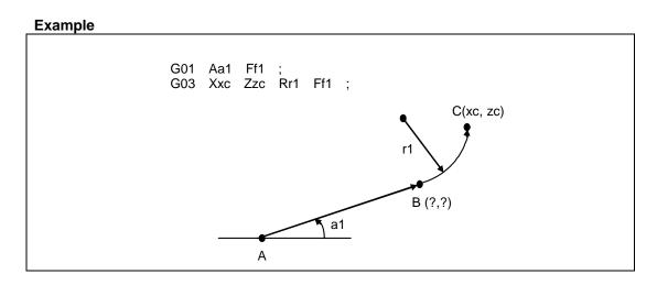
(5) Automatic calculation of arc-linear contact
