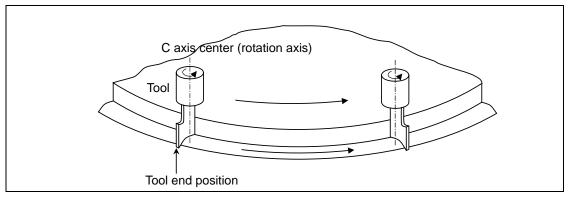
The normal line control I and II can be used according to the C axis turn direction during normal line control. This is set by the parameters.
