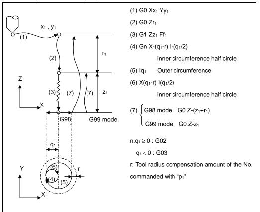
The operation stops at after the (1), (2) and (6) commands during single block operation.
