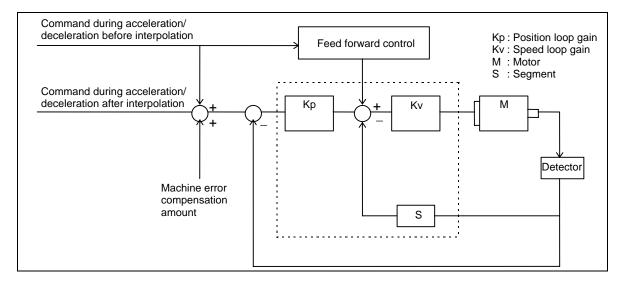
(2) Reduction of arc radius reduction error amount using feed forward control With the high-accuracy control, the arc radius reduction error amount can be greatly reduced by combining the pre-interpolation acceleration/deceleration control method above-mentioned and the feed forward control/SHG control.
