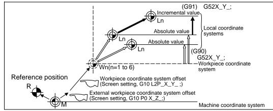
(Note) If the program is executed repeatedly, the workpiece coordinate system will deviate each time. Thus, when the program is completed, the reference position return operation must be commanded.
