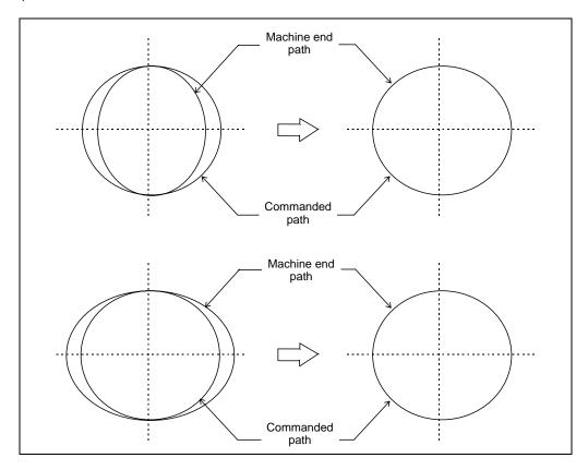
(2) Smooth compensation at entrance and exit The compensation amount is gradually increased from the arc start point to the 90° position, and 100% compensation is reached at the 90° position. The compensation is gradually decreased from 90° before the end point, and 0% compensation is reached at the end point.
