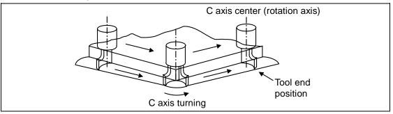
During arc interpolation, the rotation axis turning is controlled in synchronization with the operation of arc interpolation.
