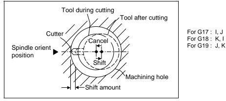
The shift amount is executed with linear interpolation, and the feed rate follows the F command.
