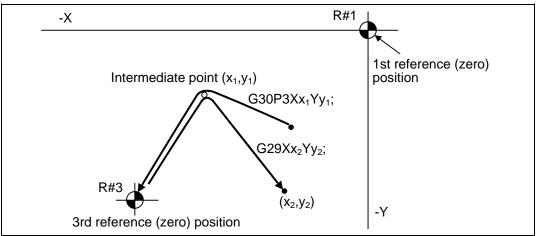
(5) With reference (zero) position return on a plane during compensation, the tool moves without tool radius compensation from the intermediate point. With a subsequent G29 command, the tool moves with tool radius compensation until the G29
