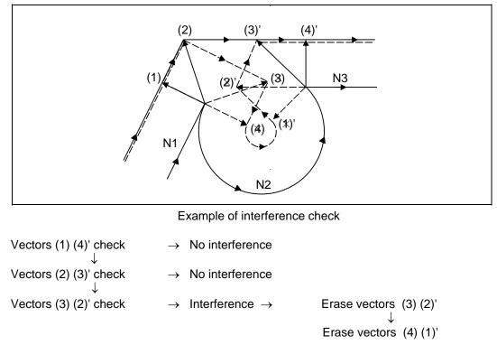
With the above process, the vectors (1), (2), (3)' and (4)' will remain as the valid vectors, and the path that connects these vectors will be executed as the interference avoidance path.
