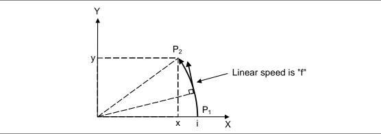
In this case, the feed rate of the X and Z axes will change along with the tool movement. However, the combined speed will always be maintained at the constant value "f".
