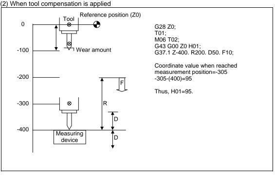
(Note) A measurement for the wear amount is applied when the current tool length compensation amount is other than zero. Thus, length wear will be compensated if length dimension by tool compensation memory type and length wear are differentiated. If not differentiated, length dimension will be compensated.
