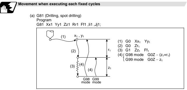
The operation stops at after the (1), (2) and (4) commands during single block operation.
