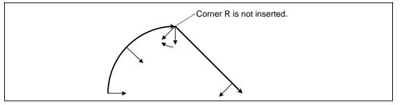
During the radius compensation, the radius compensation is applied to the path that the corner arc is inserted into.
