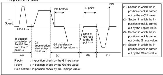
(2) Relation between the in-position width and tap axis movement for a synchronous tap in-position check
