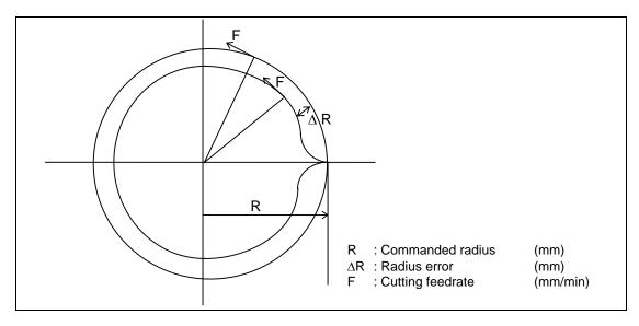
The compensation amount of the circle radius reduction error ( $\Delta R$ ) is theoretically calculated as shown in the following table.
