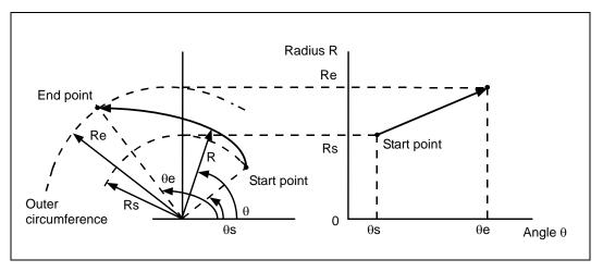
Although the speed of the outer circumference is slightly faster than the commanded speed, the angular speed is constant.
