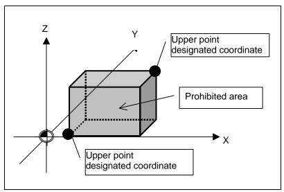
(Note) The upper point and lower point are commanded with coordinate on the machine coordinate system.
